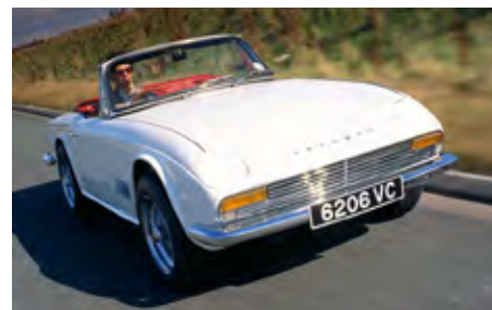
1967 / 'ZEST' prototype #2 reg. 6206 VC. Although well liked by Triumph management, Zest in this form would never make it into production as proposed US safety legislation threatened to outlaw concealed headlights.
