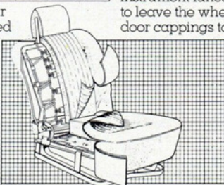
Seat design - rubber strapping, diaphragm and thick foam - greater comfort, less fatigue.
