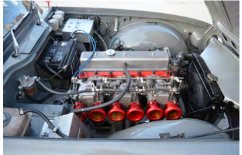
Above – TR6 fitted with a 2.6 L engine and three double Weber
