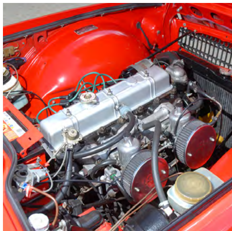
The 2.5-l inline 6 engine of a carburetted TR6
